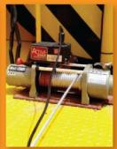
Use the remote to activate electric winch to apply winch traction. Pull the sewer cleaning debris basket in the sewer, which will be able to bringing debris in the sewer to the bottom of the manhole.
